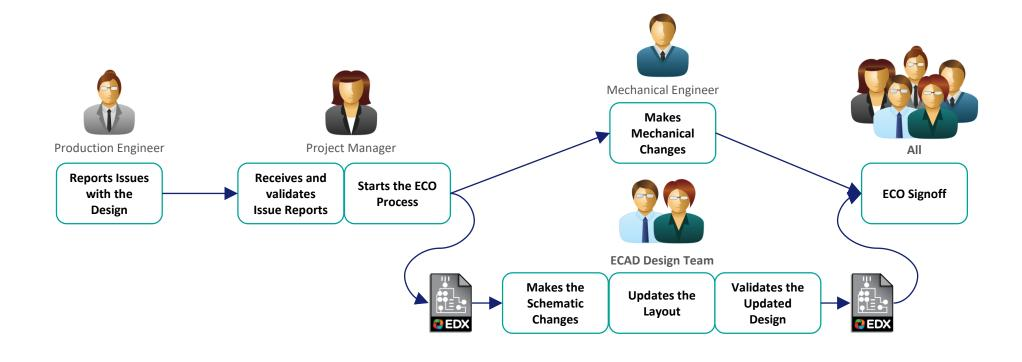
An ECAD workflow typically represents the steps within the enterprise workflow that represent the PCB design tool interactions.
