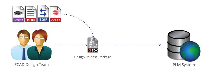
The Design Engineer creates a Design Release Package and sends it to the PLM System. The PLM System archives the EDX Package and extracts the data required to integrate it into the product structure.
