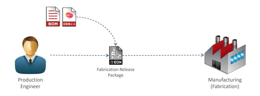
The Production Engineer prepares the product model for Manufacturing and creates the Fabrication Release Package.
