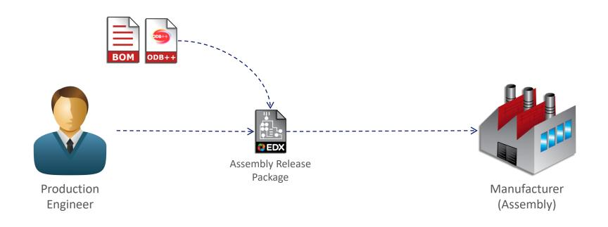
The Production Engineer prepares the product model for Manufacturing and creates the Assembly Release Package.
